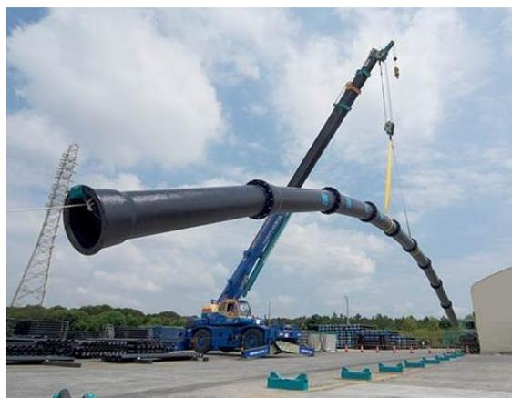
[耐震管の吊上げ実験の様子]
